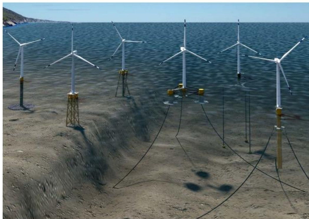
Figure 3.3. Six different offshore wind substructure types. The three on the far left are fixed-bottom substructures (monopile, jacket, and inward battered guide structure [also known as a twisted jacket]), and the three on the right are floating substructures (from left to right: semisubmersible, tension leg platform, and spar). Illustration by Josh Bauer, NREL.
